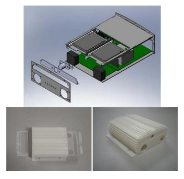
Figure 13: HDs drawer configuration and plastic prototype (0.03 scale).
