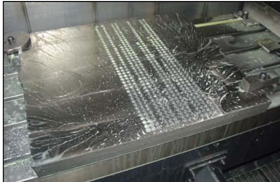
Figure 4. Workpiece used in drilling operations for tool-wear evaluation
