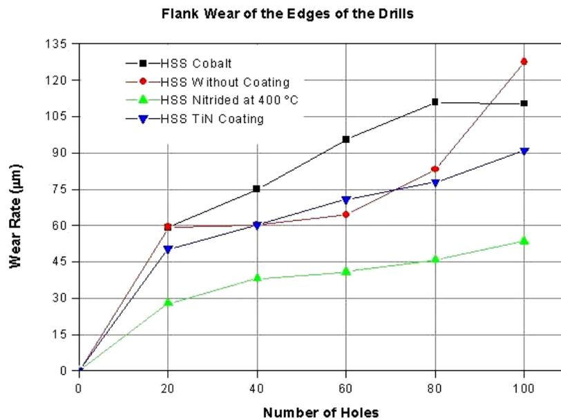
Figure 9. Comparative graph of the flank wear behavior of twist-drill cutting edges
