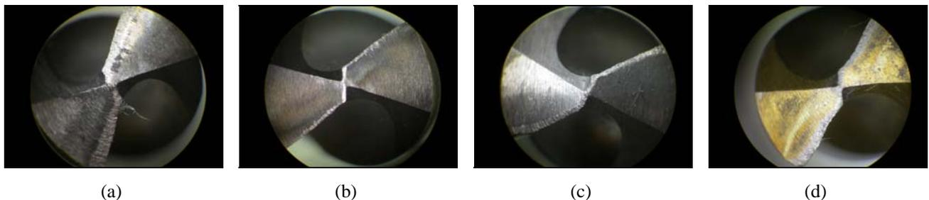
Figure 8. Photos of the main cutting edge of twist-drills after 100 holes: (a) HSS without coating; (b) HSS nitrided at 400°C; (c) HSS cobalt; (d) HSS TiN coating
