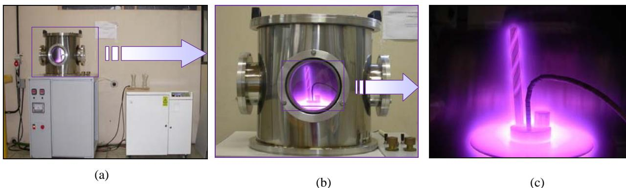
Figure 2. (a) Equipments for twist-drills plasma nitriding. (b) Plasma nitriding reactor in operation. (c) Details of instrumentation
