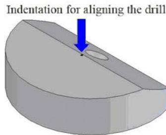
Figure 6. Tool-support scheme for positioning of twist-drills for image acquisition
