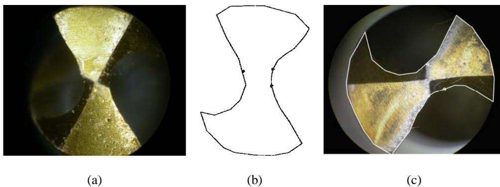
Figure 7. Photos of TiN coated HSS twist-drill: (a) new cutting edge; (b) template of cutting edge; (c) failure cutting edge with template
