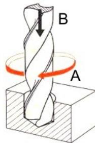
Figure 1. Drill movements in hole-making: A) cutting in rotation; B) feed in translation
