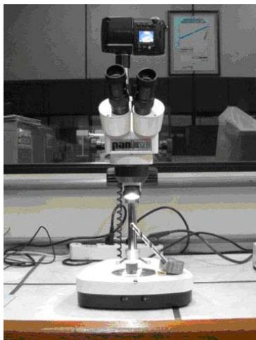
Figure 5. Digital image acquisition system for tool-wear detection through the drilling operations
