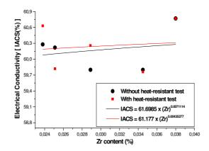
Figure 9. Comparison of IACS results without and with heat-resistant test, without aging.
