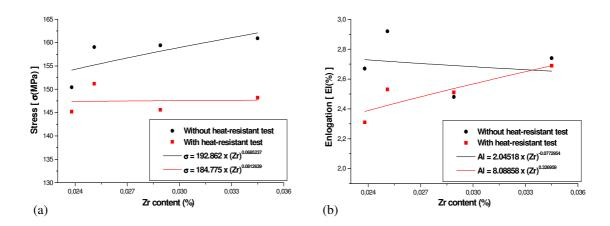
Figure 8. Comparison of results of (a) stress and (b) elongation without and with heat-resistant test, with natural aging of 1.5 year.
