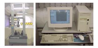
Figure 6. KRATOS, model IKCL1-USB and data acquisition system.
