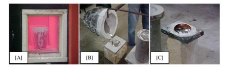
Figure 1. Photos illustrating a crucible in the oven; the collection of samples for chemical analysis and sample collected.
