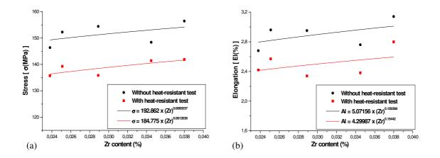
Figure 7. Comparison of results of (a) stress and (b) elongation without and with heat-resistant test, without natural aging.
