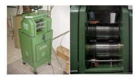
Figure 3. Electrical rolling mill utilized.
