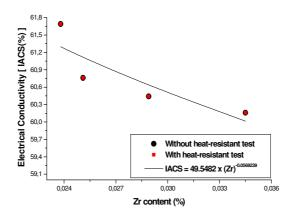
Figure 10. Results of IACS without and with heat-resistant test, with 1.5 year natural aging.
