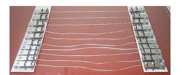
Fig. 2 A sample of HMPE creep specimens
