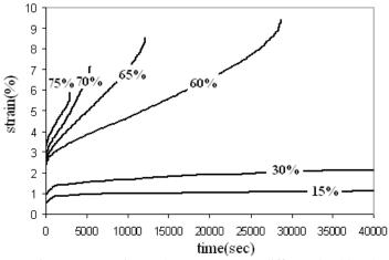
Figure 5: Experimental creep curves at different load levels.
