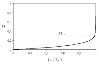
Figure 7: Damage evolution in a typical creep test.
