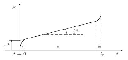
Figure 6: Typical experimental creep curve
