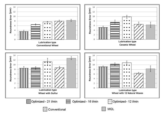
Figure 3. Roundness error versus lubrication type
