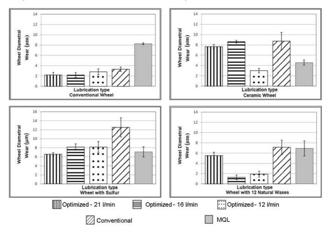
Figure 4. Diametral wheel wear versus lubrication type
