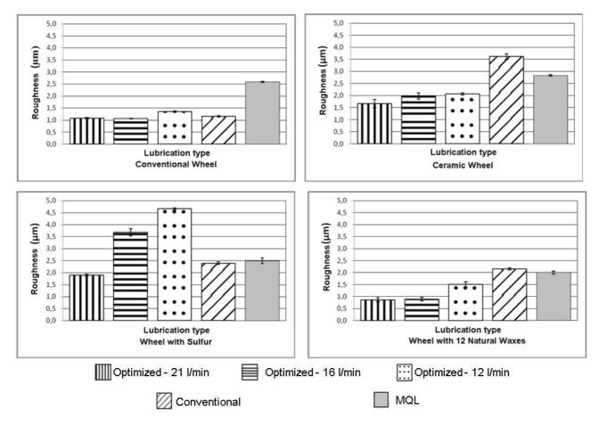
Figure 2. Roughness versus lubrication type
