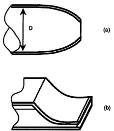
Figure 1. Optimized (a) and conventional (b) shape nozzles
