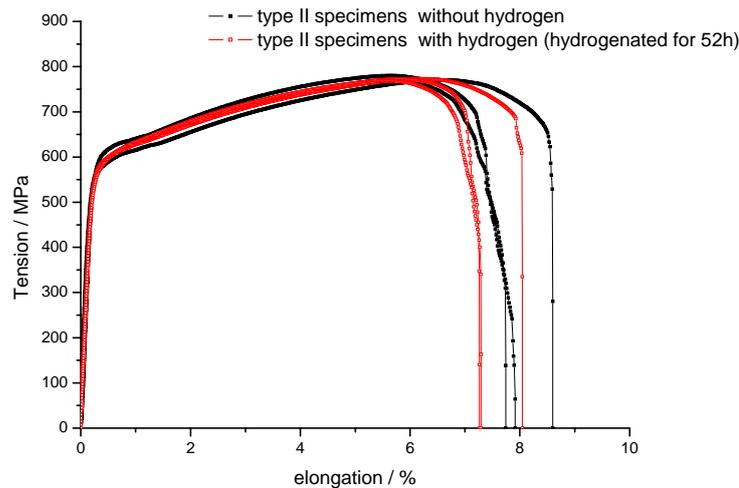
Figure 5. Stress–strain curves plotted for API 5L X60 steel Type II without hydrogen (black points) and with hydrogen charged for 52 h (red points).
