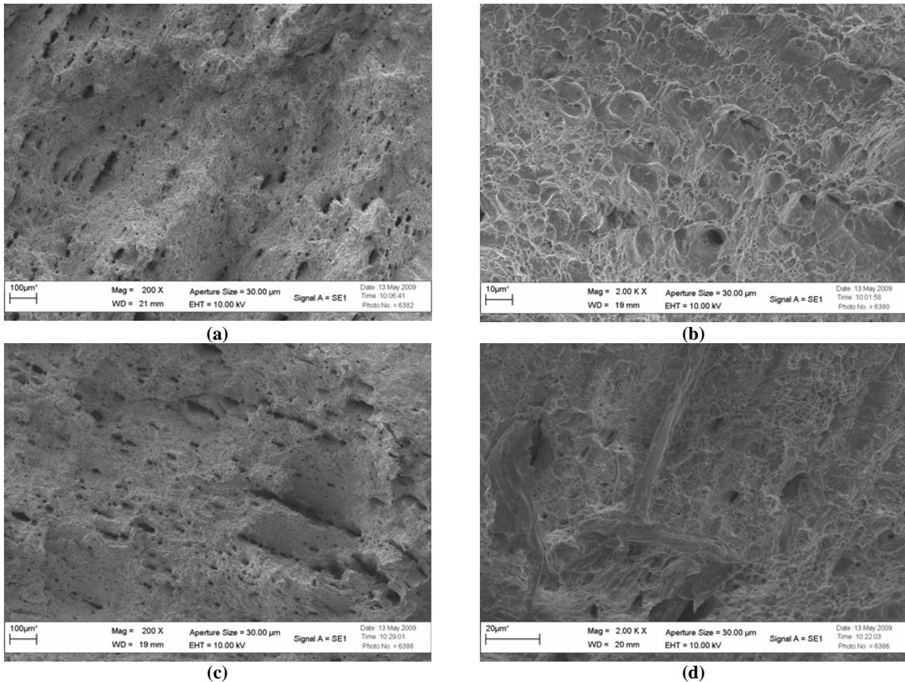
Figure 6. SEM of fracture surface of API 5L X60 steel Type I: (a) without hydrogen. 200X, (b) without hydrogen. 2000X; (c) with hydrogen. 200X and (d) with hydrogen. 2000X.
