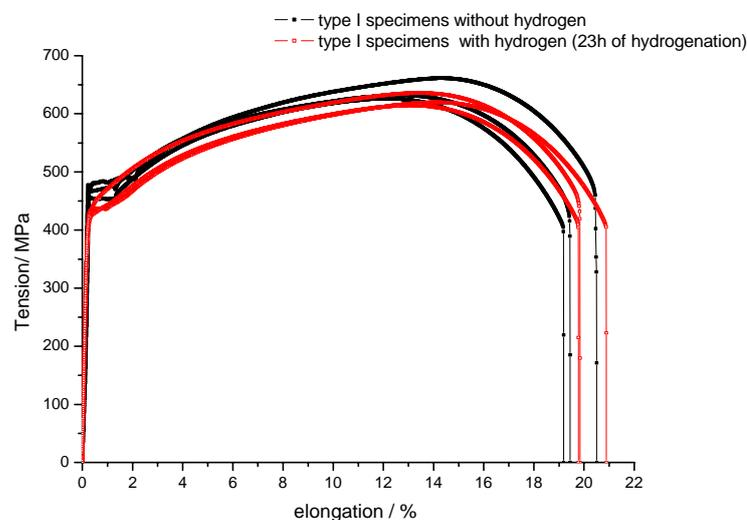
Figure 4. Stress-strain curves plotted for API 5L X60 steel Type I without hydrogen (black points) and with hydrogen charged for 23 h (red points).
