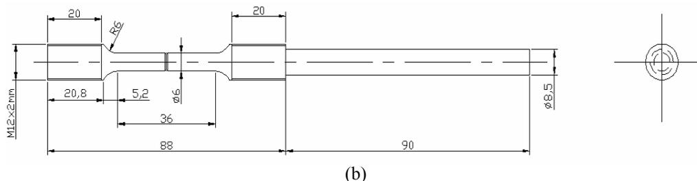
Figure 1. Geometry and dimensions (in mm) of the specimens. (a) Type I to reproduce environmental hydrogen (EHE) and (b) Type II to reproduce internal hydrogen embrittlement (IHE).
