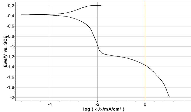
Figure 3. Potentiodynamic polarization for API 5L X60 steel.
