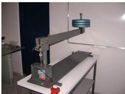
Figure 2. Fixture used for the hydrogenation process in IHE (Costa, 2008)
