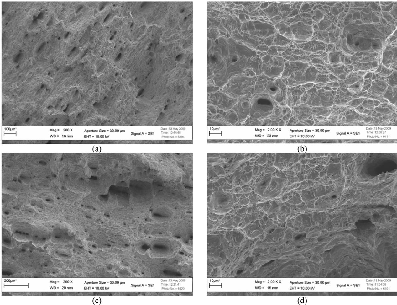
Figure 7. SEM of fracture surface of API 5L X60 steel Type II: (a) without hydrogen. 200X, (b) without hydrogen. 2000X, (c) with hydrogen. 200X and (d) with hydrogen. 2000X.
