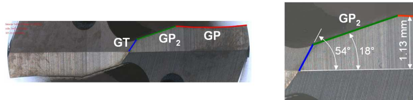
Figure 4. Type A relief sharpening of the chisel edge
