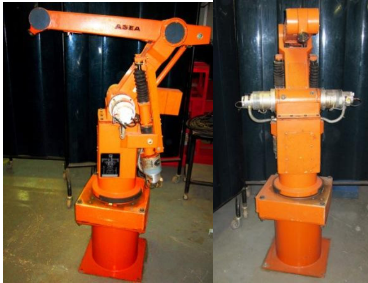
Figure 14. Five axes robot, ASEA, used in the experiments.
