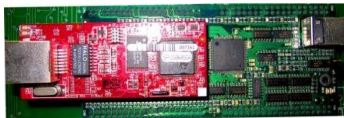
Figure 4. Grex G100 Pulse Generator.
