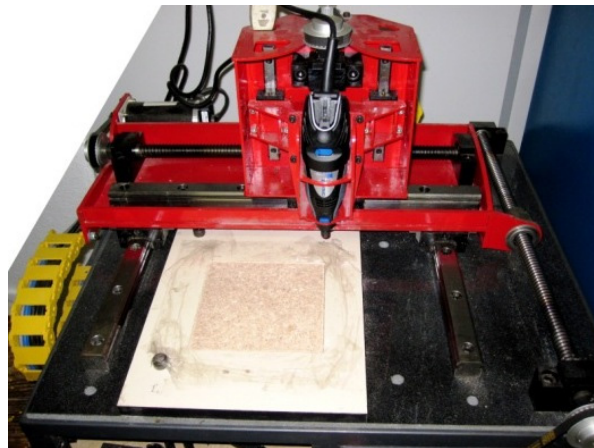
Figure 12. Small Scale Mill with controller developed in same methodology.
