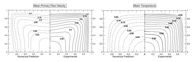
Figure 5. Streamwise velocity contours  $U/U_C$  (a); Mean Temperature  $(T_W-T)/(T_W-T_C)$  (b)
