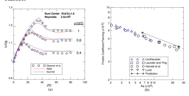
Figure 2. Axial mean velocity distributions at various streamwise locations (a); Friction coefficient for fully developed flows in a square duct (b)
