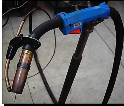
Figure 3. Wire feeding device connected to the welding torch.
