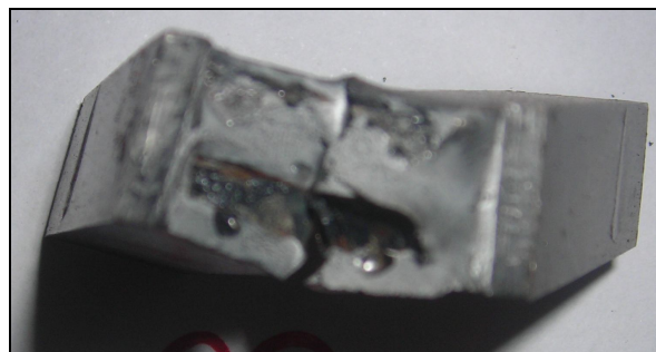
Figure 16. MAG-CW Charpy specimen after the Impact Strength Test.
