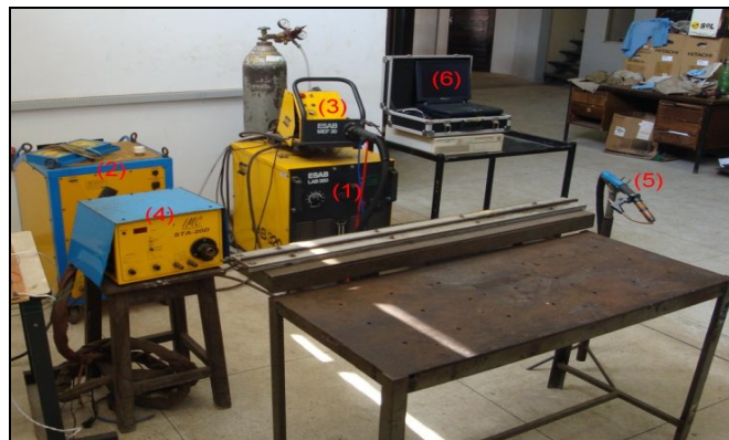
Figure 2. Welding bench used in the welding deposition. (1) Welding power source; (2) Auxiliary power source; (3) Auxiliary wire feeding welding head; (4) Auxiliary cold wire welding head; (5) Torch; (6) Notebook used for data purchase.
