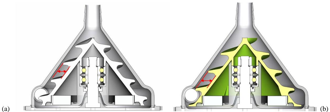
Figure 4. (a) Prototype #5 without cylindric base and increasing 0,7 mm at the thread deep and (b) Prototype #6 with cylindric base and increasing 1,2 mm at the thread deep.
