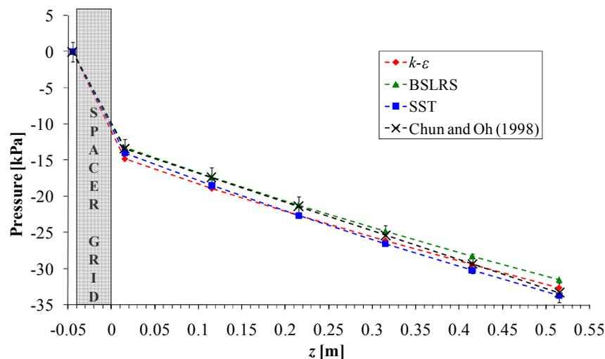
Figure 10. Pressure loss along the rod bundle
