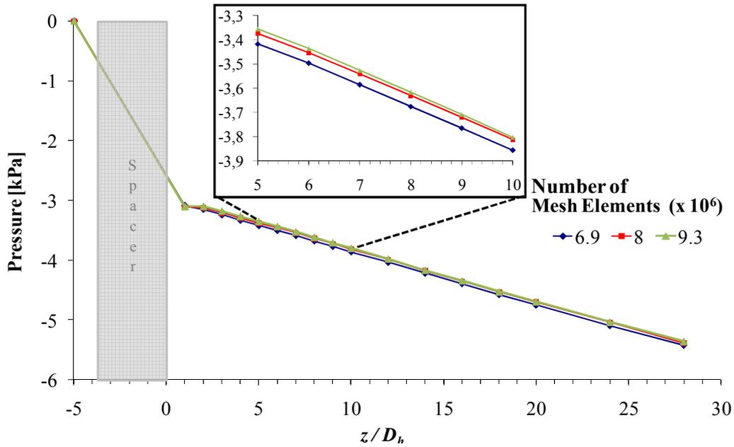
Figure 4. Pressure profiles for different meshes
