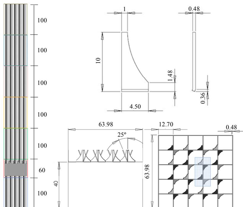
Figure 1. Computational domain of the simulations with details of the spacer grid and the vanes (units in mm)
