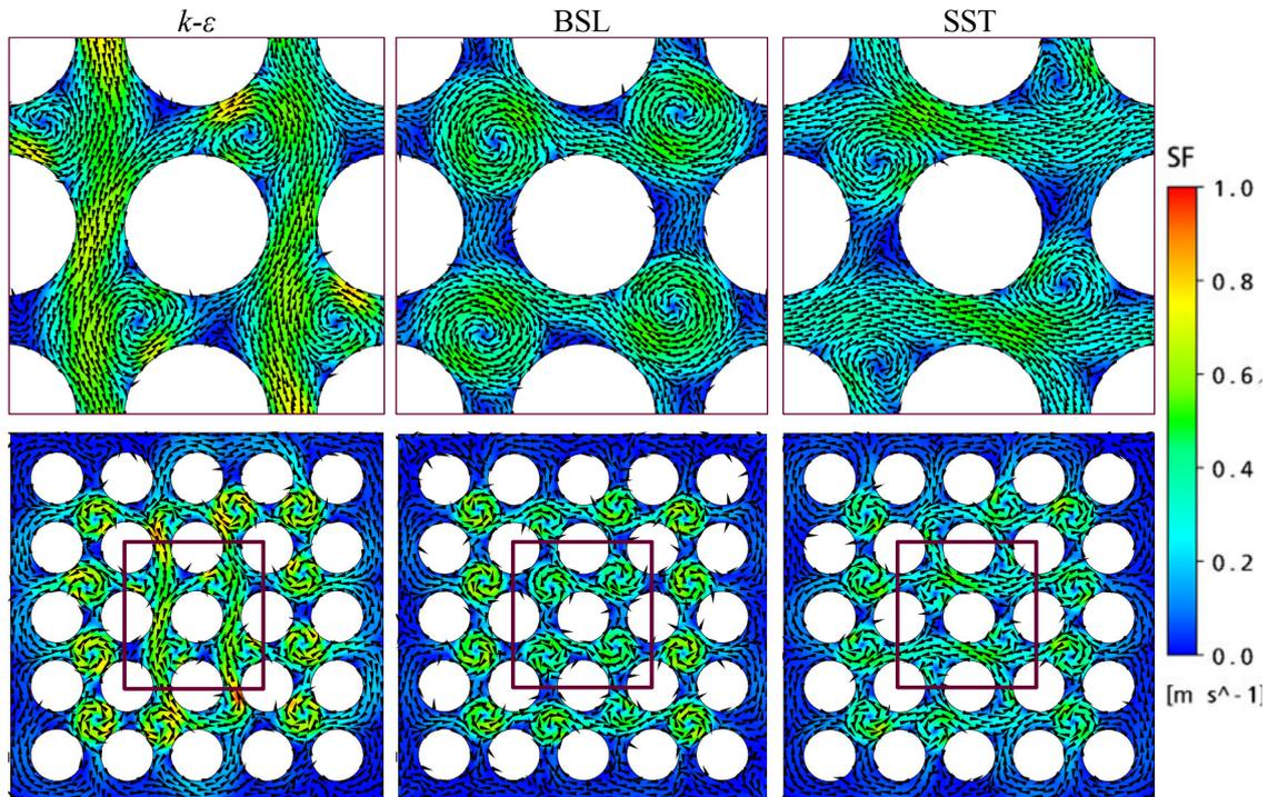
Figure 9. Velocity vectors and intensity tangent to a plane placed 463.5 mm downstream the spacer grid
