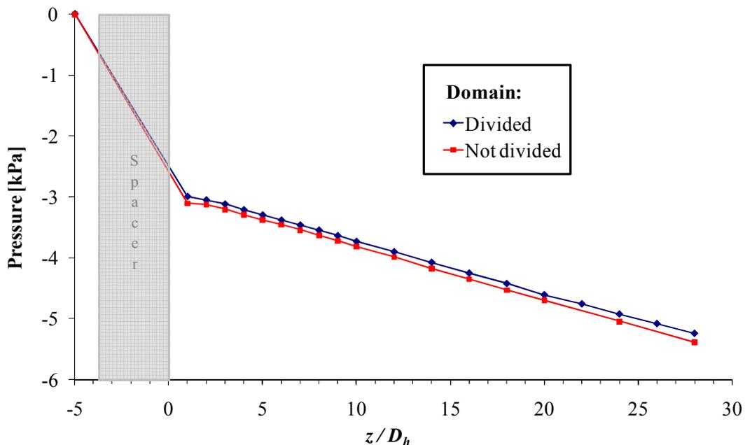
Figure 3. Pressure profiles downstream the spacer grid without and with the domain division
