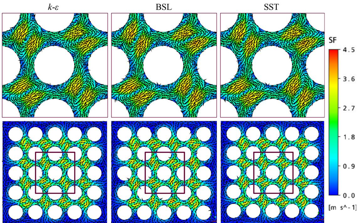
Figure 8. Velocity vectors tangent to a plane placed 12.7 mm downstream the spacer grid
