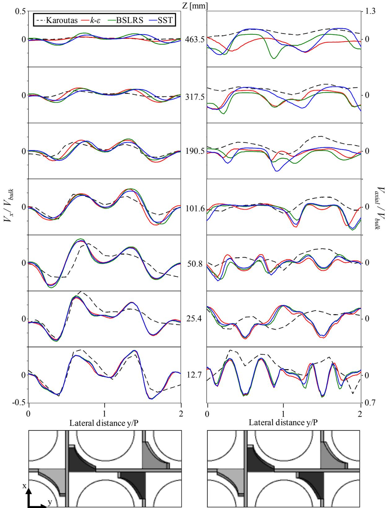
Figure 6. Lateral and axial velocity profiles downstream the spacer grid
