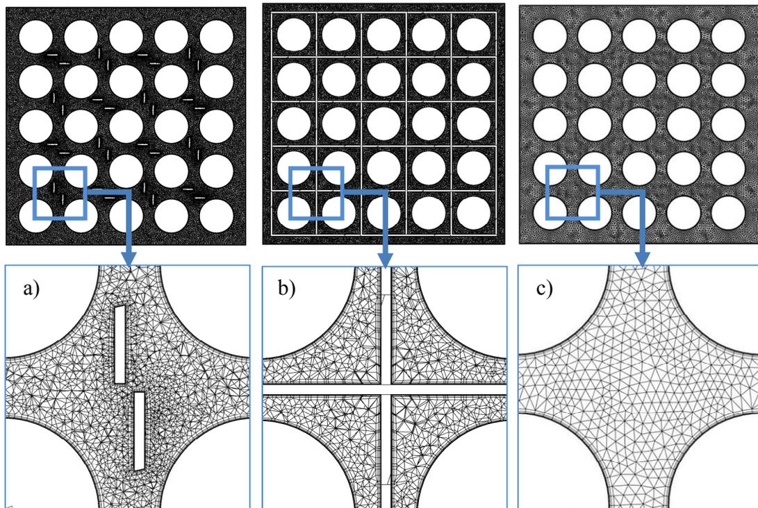
Figure 5. Mesh cross section in the vane (a), grid (b) and bare bundle (c) regions
