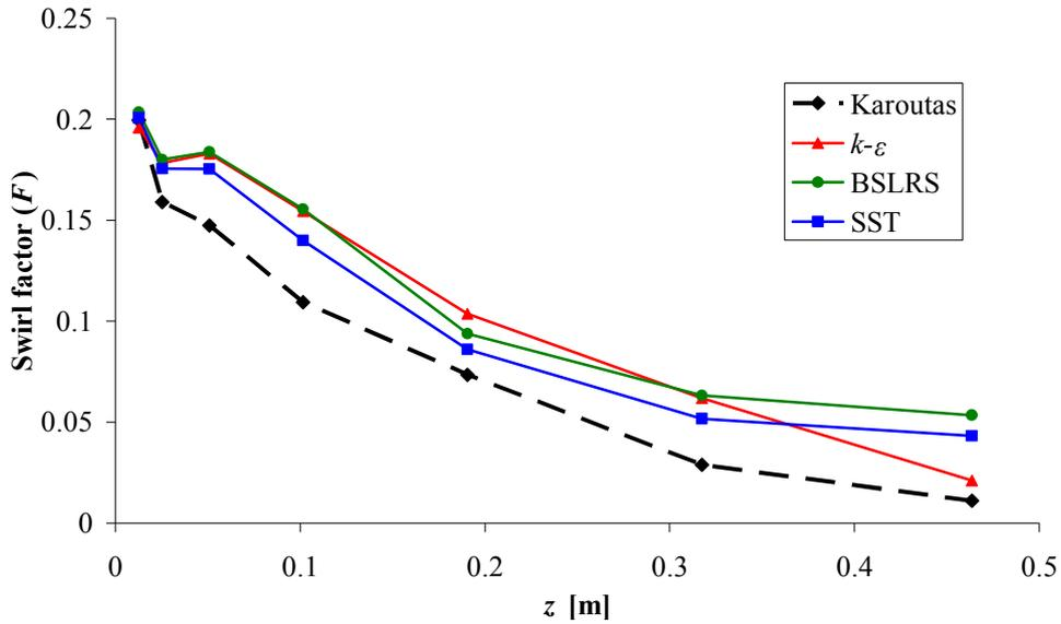
Figure 7. Swirl factor downstream the spacer grid
