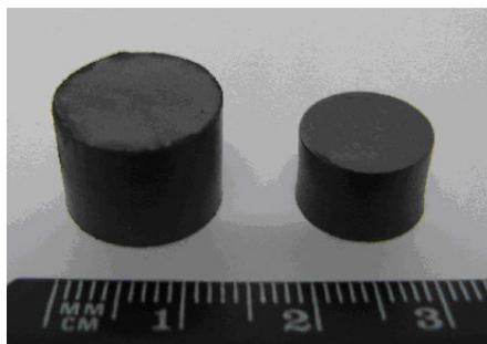
Figure 7: 1st sample sintered 2nd sample compacted WC20-Co
