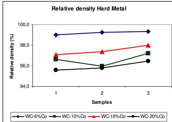
Figure 5: Relative density of hard metal composites
