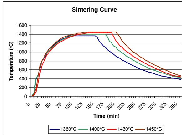
Figure 4: Sintering curve dos hard metal composites
