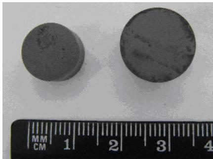
Figure 6: 1st sample sintered and 2nd sample compacted WC15-Co
