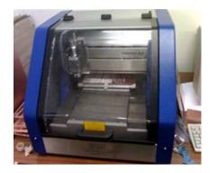
Figure 6. Example of a low cost CNC milling machine, used for milling PCBs
