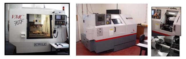
Figure 5. Modern CNC machines accept numerical instructions to control its moving elements; A NC machining center (left), and a lathe (middle); Top right- lathe's protection door opened showing the tools and the part; Bottom right – blank material and tool, ready to the operation start.
