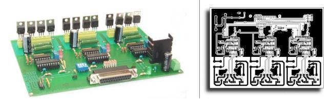
Figure 9. CNC3AX board and the printed circuit map – controls up to 3 step motors (FEOGA).
