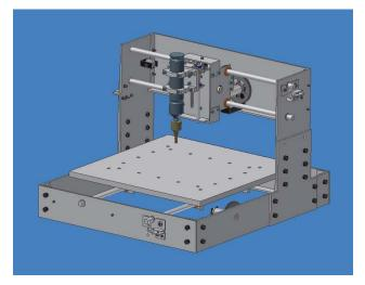
Figure 11. 3D CAD model of the CNC milling machine under development at the UMinho.
