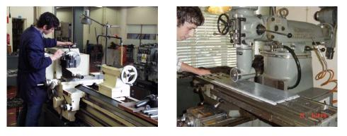
Figure 1. Conventional manufacturing operations in a lathe (left) and a in a milling machine (right); Skilled professionals are needed to handle the machines, and risk is all time present.
