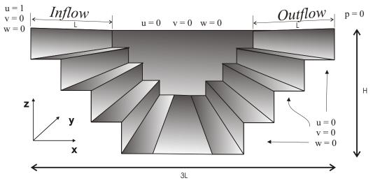
Figure 2. Perspective on y axis e boundary conditions for the simulation using stairs on reservoirs.
