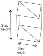
Figure 3. Detail of the dimension of a stair step.
