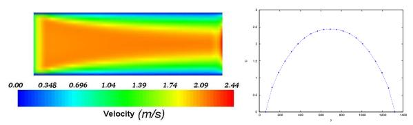
Figure 5. Simulation in a stair steps domain, field of velocity component in direction x with Re = 100, with five layer of prisms.
