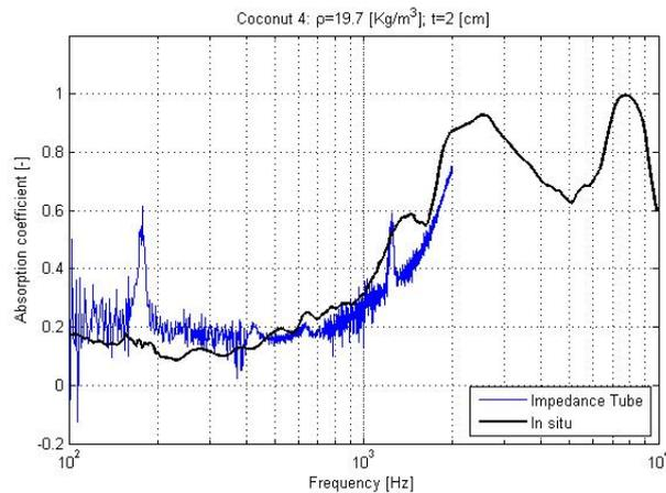
Figure 8. Absorption coefficient of coconut material 4 (Impedance tube vs. *In situ*).
