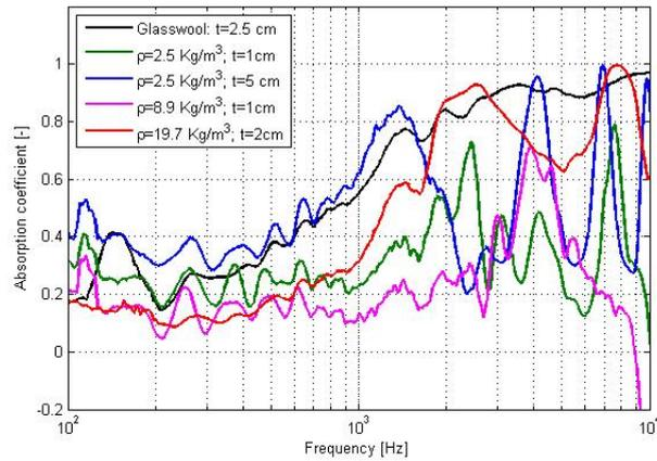
Figure 9. Absorption coefficient of all materials tested with the *in situ* technique.
