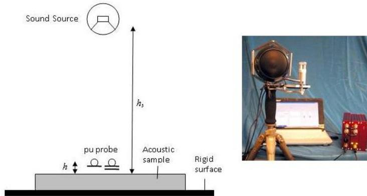
Figure 2. The impedance setup.
