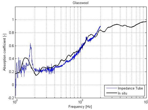
Figure 3. Absorption coefficient of glass wool (Impedance tube vs. *In situ*).
