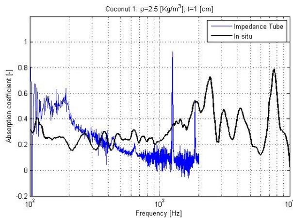
Figure 5. Absorption coefficient of coconut material 1 (Impedance tube vs. *In situ*).
