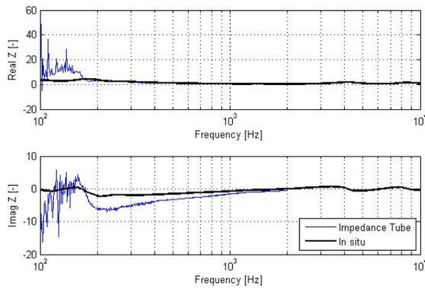
Figure 4. Surface impedance of glass wool (Impedance tube vs. *In situ*).
