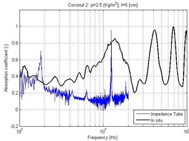
Figure 6. Absorption coefficient of coconut material 3 (Impedance tube vs. *In situ*).
