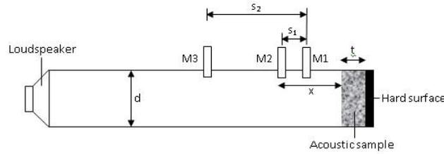
Figure 1. Impedance tube schematic drawing
