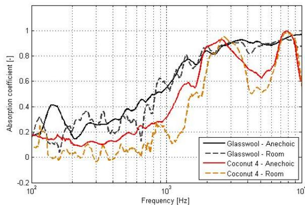
Figure 10. Absorption coefficient of glasswool and coconut 4 measured in the semi anechoic room and in a regular room.
