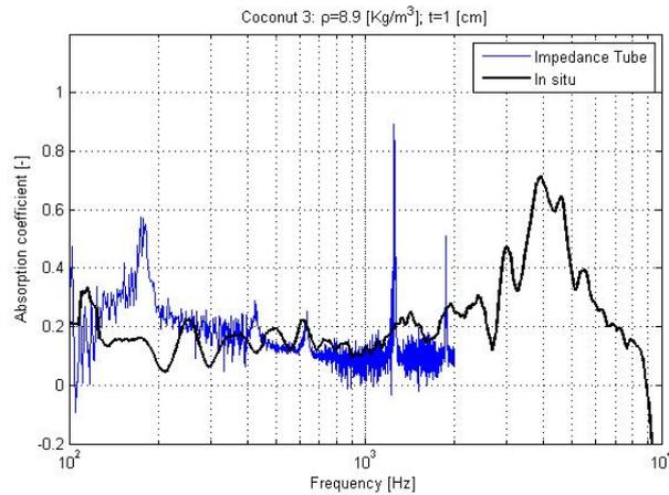
Figure 7. Absorption coefficient of coconut material 2 (Impedance tube vs. *In situ*).
