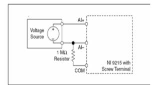
Figure 1. Connection of a floating differential voltage signal to the NI 9215 with Screw terminal
