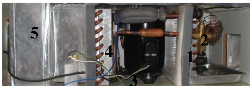
Figure 3. Heat pump from side view: (1) Evaporator, (2) Expansion Valve, (3) Compressor, (4) Condenser e (5) Fan
