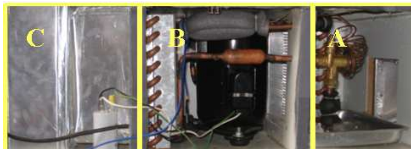
Figure 4: Heating Process: (A) Dehumidifying; (B) Heating; (C) Pumping
