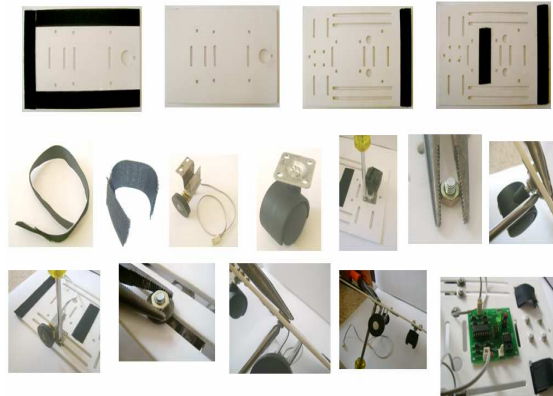
Figure 3. Second Step in the construction of the TEAC 2 H-RI kit. Base structure assembly.
