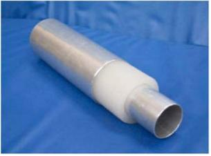
Figure 1. A sandwich pipe construction (Estefen et al (2005)).
