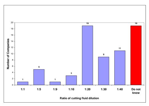
Figure 3. Ratios of dilution of cutting fluids
