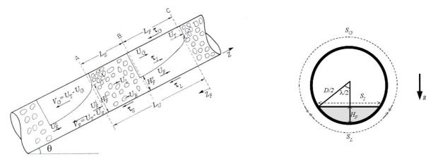
(a) Unit cell geometry. Figure 1. Schematic diagram for slug flow zones.
