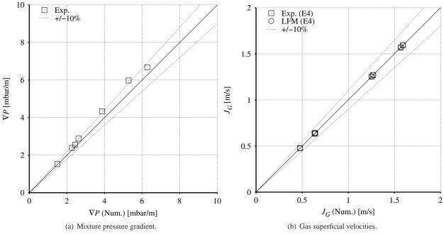
Figure 3. Comparison between experimental and numerical data.
