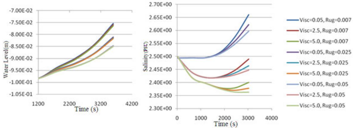
Figure 4. Results obtained with different parameter values for water free level and salinity.
