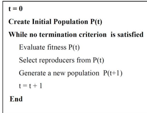
Figure 3. General structure of an Evolutionary Algorithm.
