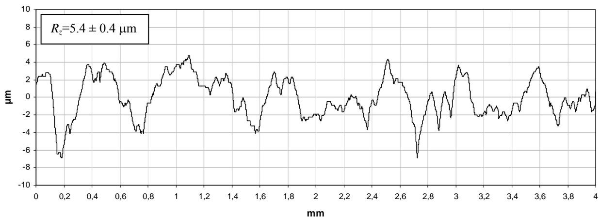
Figure 8. Profile and  $R_z$  after shot peening of specimen ground up to depth of 0.1 mm.
