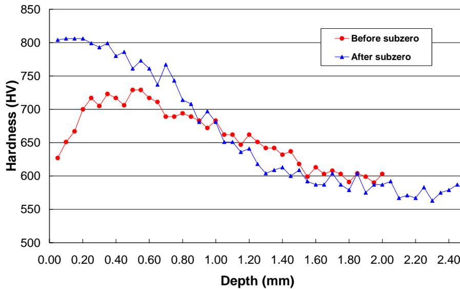
Figure 3. Microhardness profiles before and after subzero treatment.
