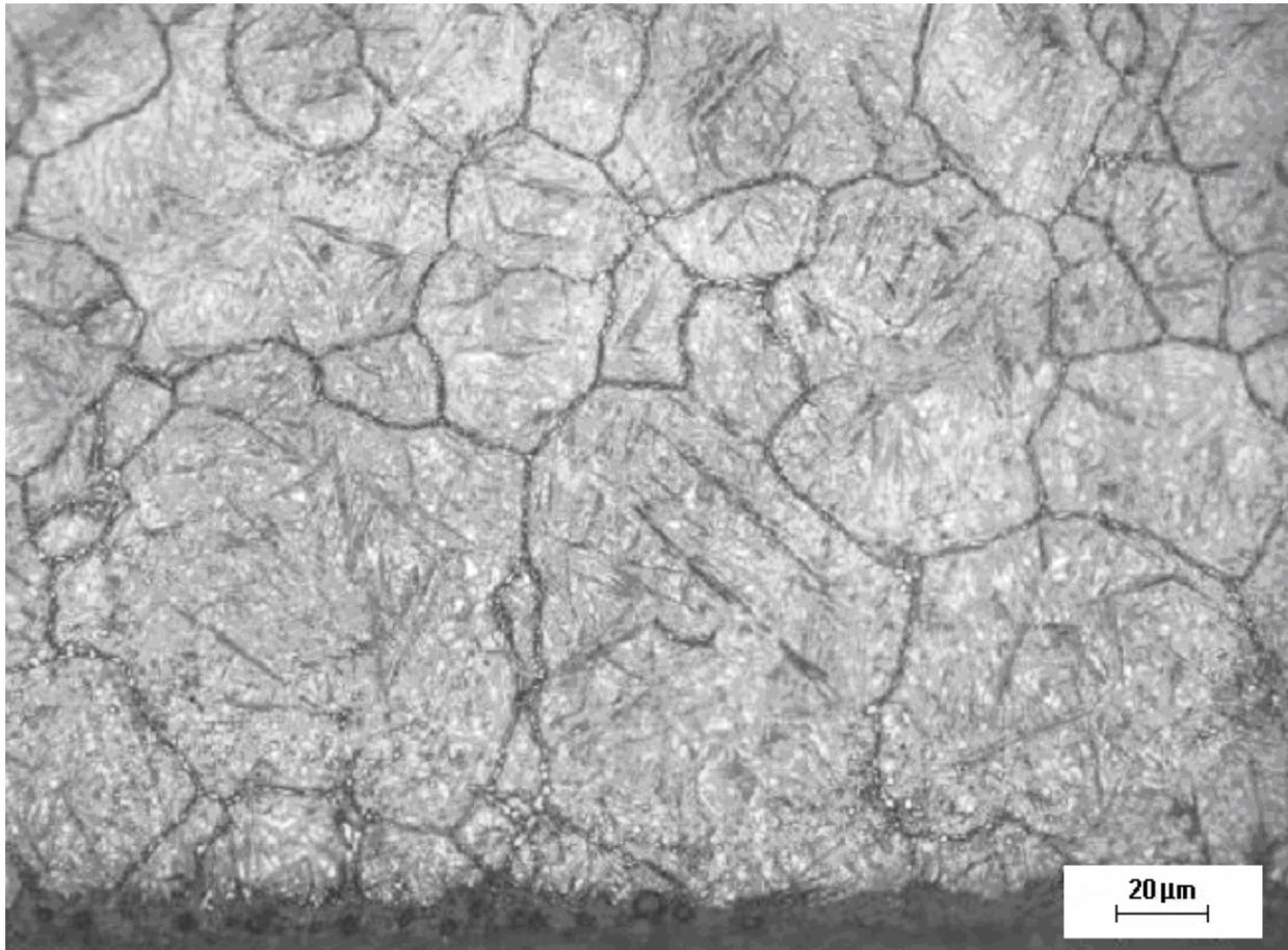
Figure 5. Surface microstructure of carburized and quenched P20 steel after subzero treatment (Nital 10%).
