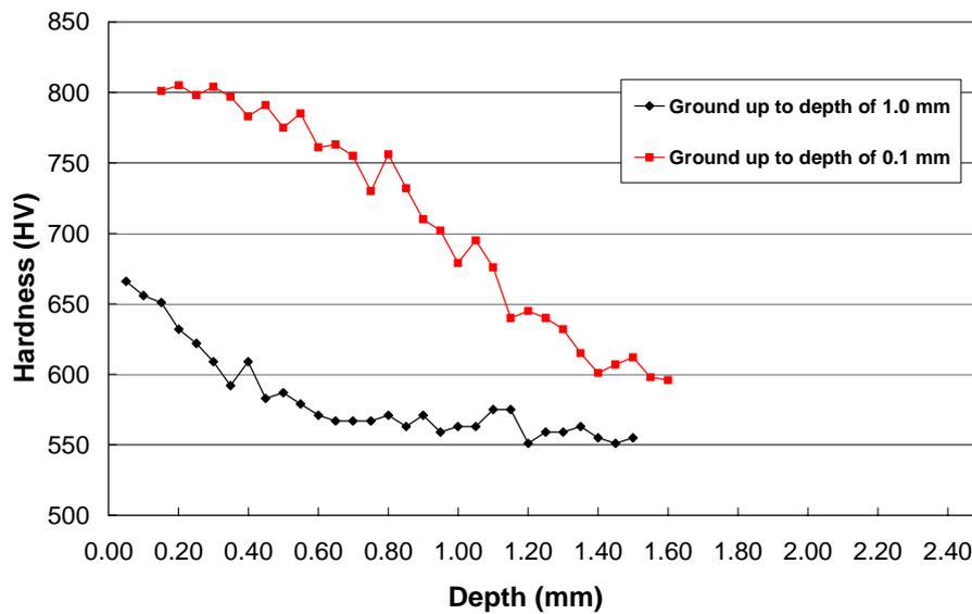
Figure 6. Microhardness profiles after two grinding levels of carburized, quenched and tempered specimens. The values of  $R_a$  roughness after grinding were 5.8 and 4.6  $\mu\text{m}$  for specimens ground up to depths of 0.1 mm and 1.0 mm, respectively.
