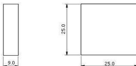
Figure 2. Dimensions (in millimeters) of the specimens after machining and grinding.
