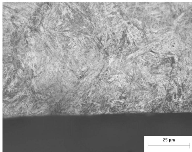
Figure 7. Microstructure of P20 steel ground up to depth of 1.0 mm after shot peening (Nital 10%).
