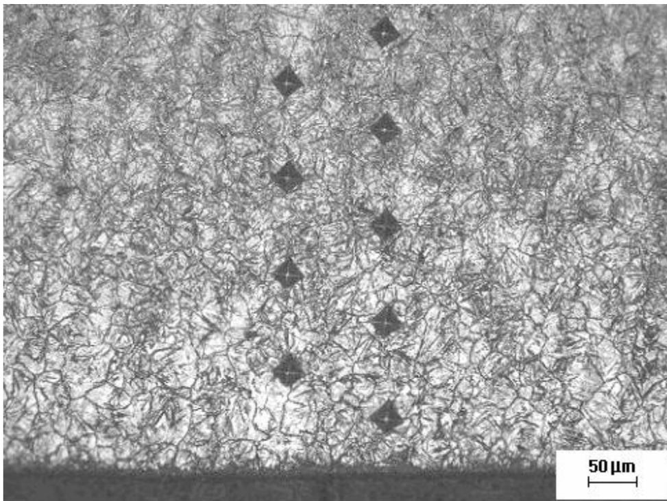
Figure 4. Surface microstructure of carburized and quenched P20 steel before subzero treatment (Nital 2%).
