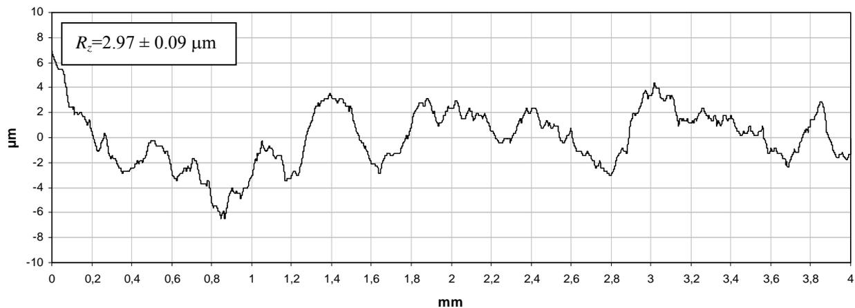
Figure 9. Profile and  $R_z$  after shot peening of specimen ground up to depth of 1.0 mm.
