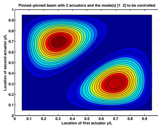
Figure 5. Controllability index for first two mode shapes of simply supported beam.
