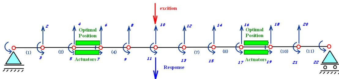
Figure 4. Beam setup with with two array of piezoelectric actuators.
