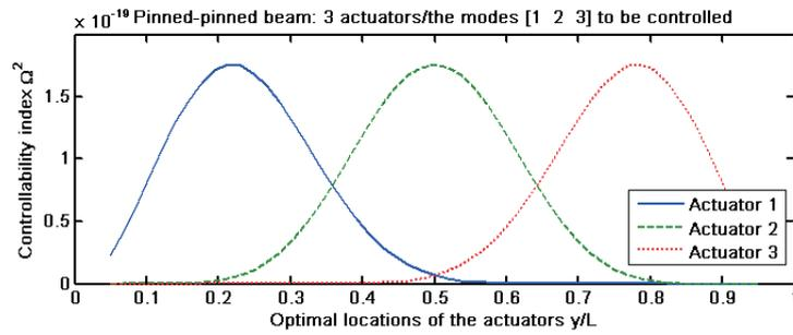
Figure 8. Controllability index for first three mode shapes of simply supported beam with three bonded actuators.
