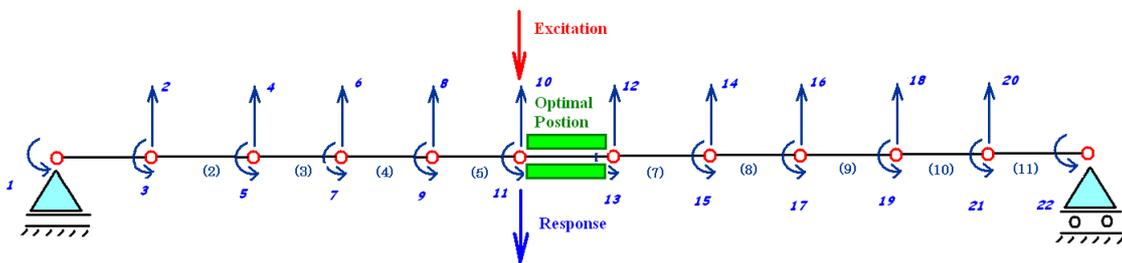
Figure 1. Beam setup with one array of piezoelectric actuators.
