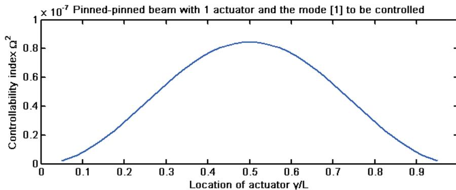
Figure 2. Controllability index for first mode shape of simply supported beam.
