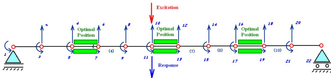
Figure 7. Beam setup with three arrays of piezoelectric actuators.
