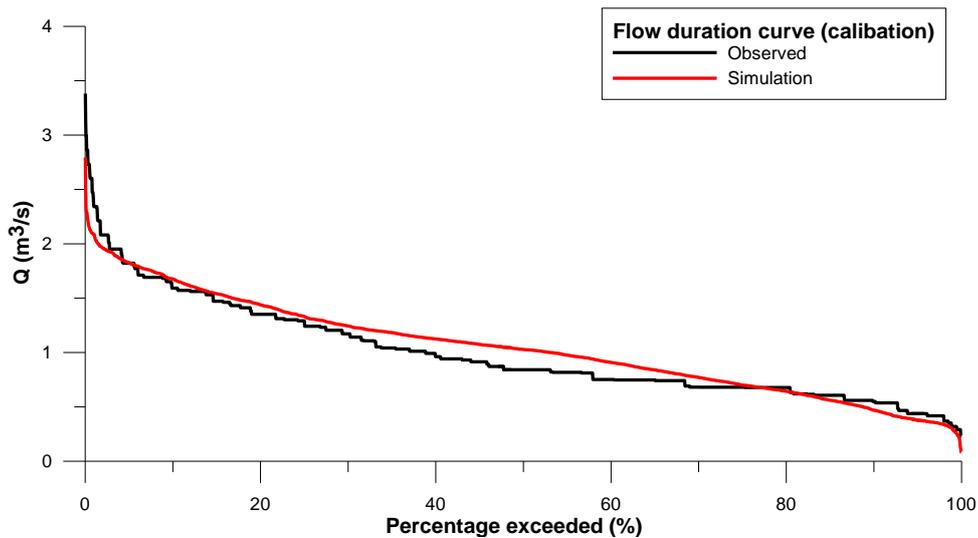
Figure 5. Flow duration curve of calibration period.
