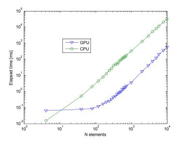
Figure 7. Time spent by the GPU and the CPU to calculate H and G.
