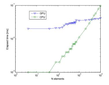
Figure 8. Time spent by the GPU and the CPU to distribute the vectors **u** and **q** among **x** and **b**', and switch the columns between **H** and **G**.
