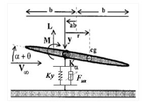
Figure 1 – 2-DOF pitching and plunging airfoil section
