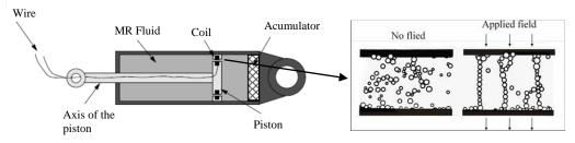
Figure 2 - Mechanical schema of MR damper and rheological behavior of MR fluid in the damper orifice.
