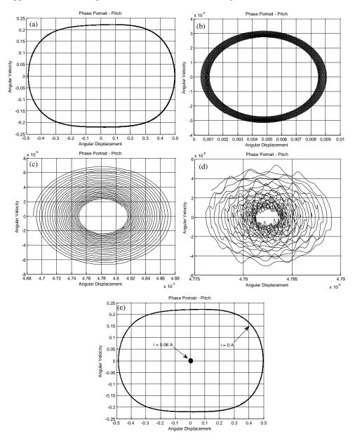
Figure 5. Evolution of Phase Portrait of Pitch degree of freedom, U = 20 m/s, (a) i = 0.4; (b) i = 0.06A; (c) i = 0.08A; (d) i = 0.1A; (e) LCO's Amplitude comparison.
