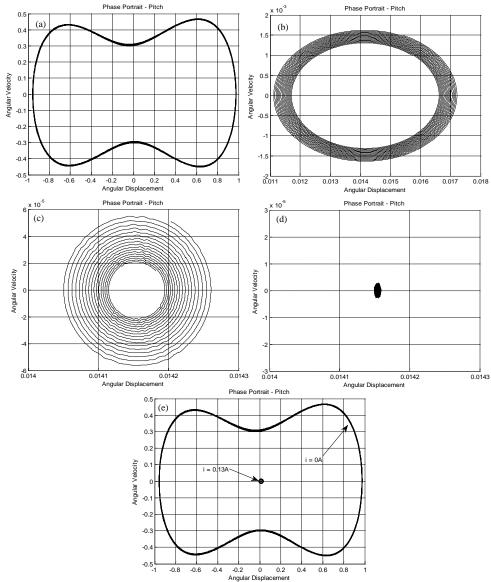
Figure 7. Evolution of Phase Portrait of Pitch degree of freedom, U = 25 m/s, (a) i = 0.4; (b) i = 0.13A; (c) i = 0.0.16A; (d) i = 0.2A; (e) LCO's Amplitude comparison.
