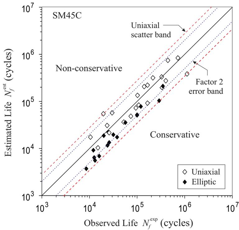
Figure 3. Estimated  $\times$  observed lives for SM45C steel (Lee, 1985).
