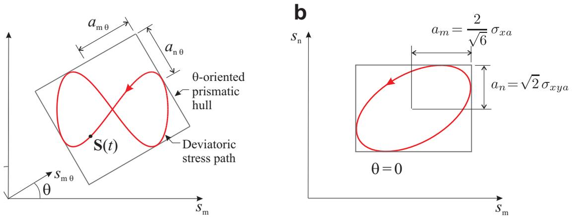
Figure 2. (a) Prismatic hull enclosing an arbitrary stress path in the deviatoric space. (b) Amplitudes  $a_m$  and  $a_n$  in the case of elliptic stress path.
