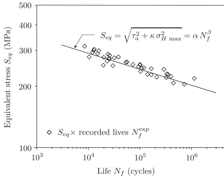
Figure 1. Generalized S-N curve using the prismatic hull as the measure of shear stress amplitude, considering bending and torsion data from Lee (1985).
