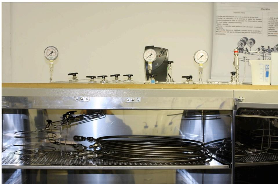
Figure 3. Slim tube test apparatus.
