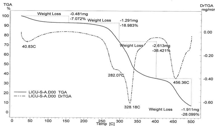
Figure 8. Thermogravimetric curve of dry licuri fiber.
