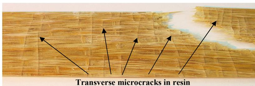
Figure 14. Transverse microcracks in the matrix – Longitudinal uniaxial tension.
