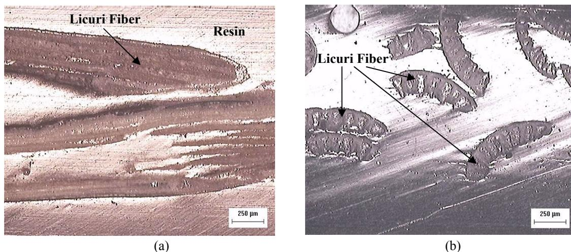
Figure 10. Composite Microstructure: (a) Longitudinal section of the lamina; (b) Transverse section of the lamina.
