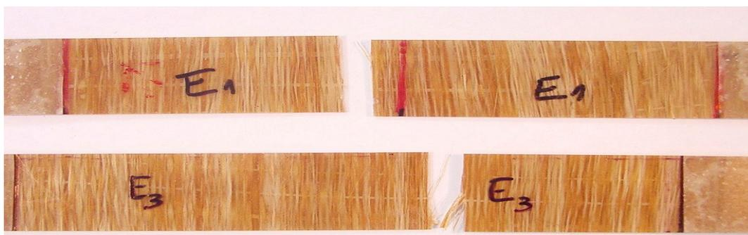
Figure 16. Flat fracture obtained in transverse uniaxial tensile tests.
