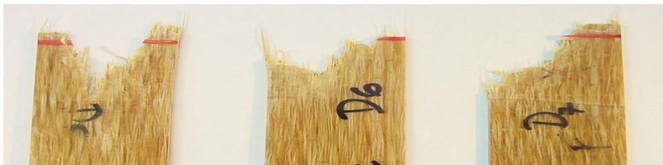
Figure 13. Different characteristics of the final fracture – Longitudinal uniaxial tensile test.
