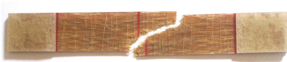
Figure 12. Longitudinal uniaxial tensile fracture in the test specimen.
