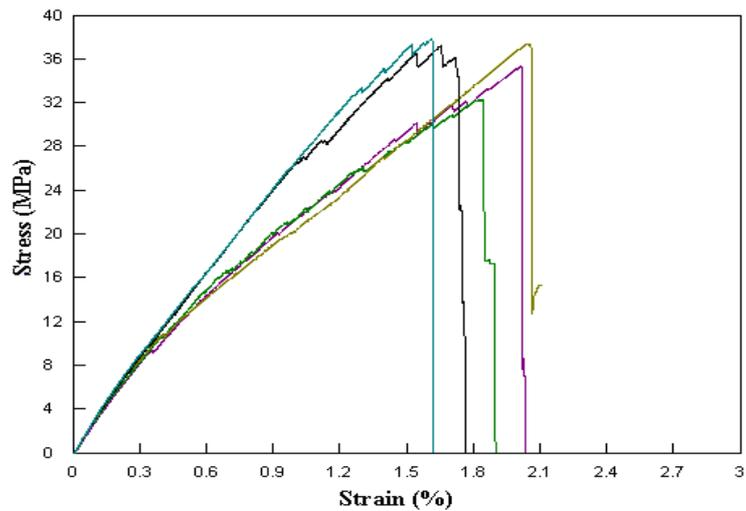
Figure 11. Stress x Strain Diagram – Longitudinal uniaxial tensile test.
