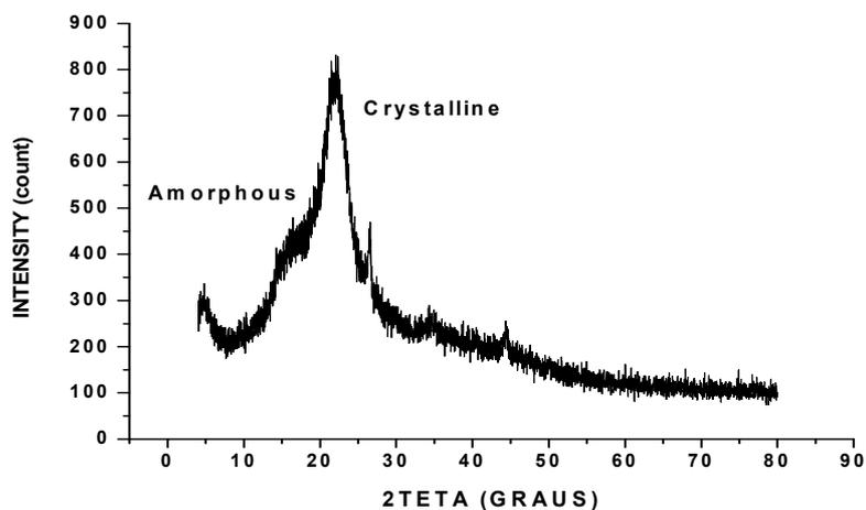
Figure 9. Diffractogram profile of the licuri fiber.
