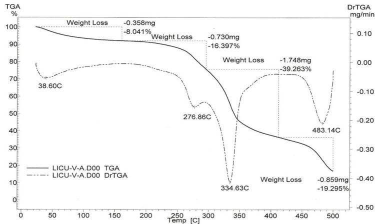
Figure 7. Thermogravimetric curve of green licuri fiber.
