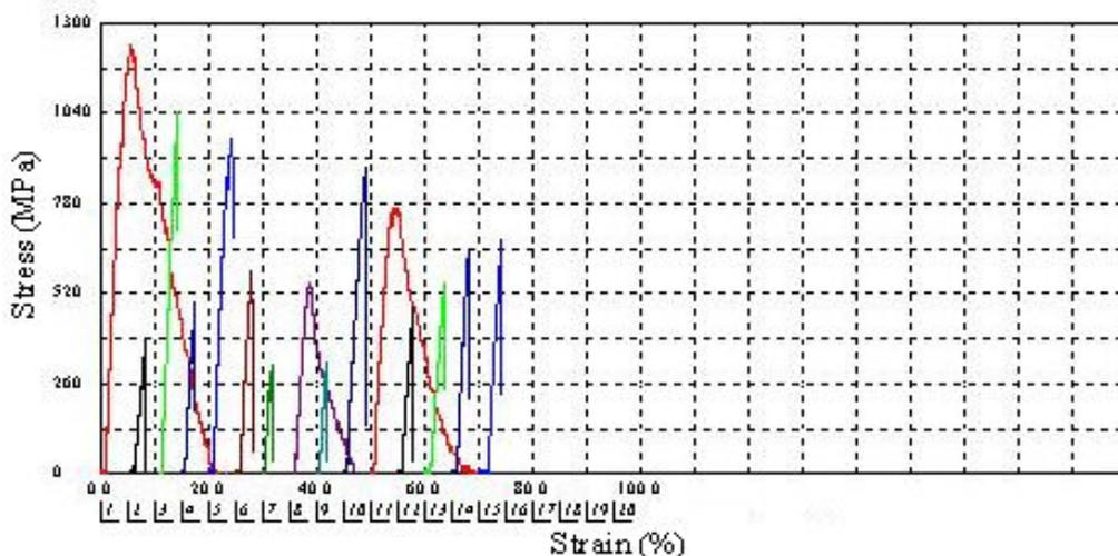
Figure 6. Stress versus strain diagram – Uniaxial tensile strength of the licuri fiber.
