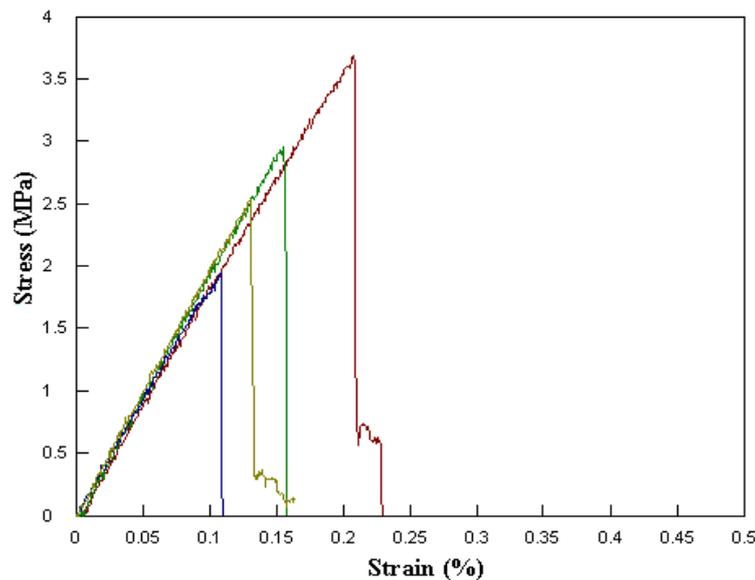
Figure 15. Stress x Strain Diagram – Transverse uniaxial tensile test.
