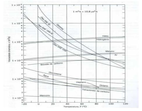
Figure 4. Diagram of viscosity versus temperature for various oils.
