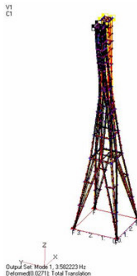
Figure 2. Bending fundamental frequency of 3.58 Hz
