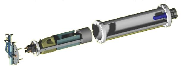
Figure 6. Details of the Tinta-P container unit and onboard components.
