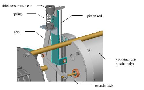
Figure 7. Details of the Tinta-P container unit and onboard components.
