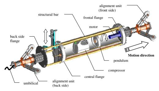
Figure 5. Details of Tinta-P components.
