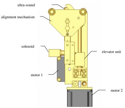
Figure 2. First prototype: mechanism main parts.
