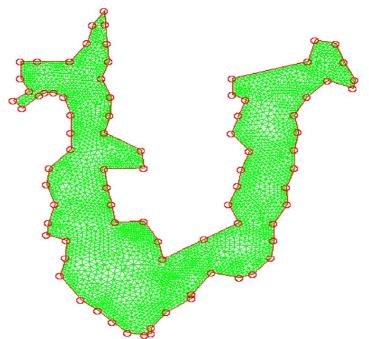
Figure 5 – Hydrodynamic mesh of Água Prtea Lake.
