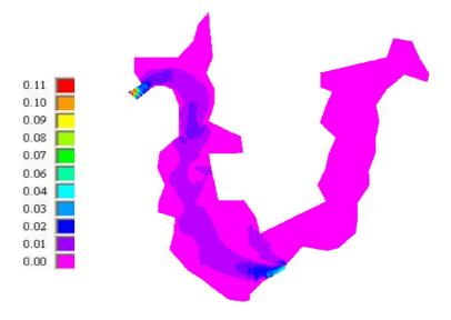
Figura 8 – Simulated Velocity Modulus Field (m/s).
