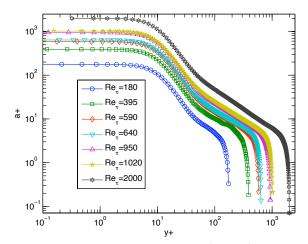
Figure 1. The profiles of velocity gradient  $a^+$  vs.  $y^+$  in log-log plot.
