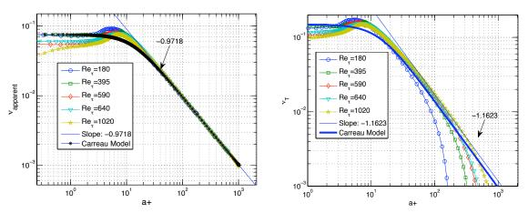
Figure 2. The profile of apparent viscosity  $\nu_{apparent}$  (a) and turbulent viscosity  $\nu_T$  (b) vs. shear rate  $a^+$  in log-log plot and Carreau model fitting.
