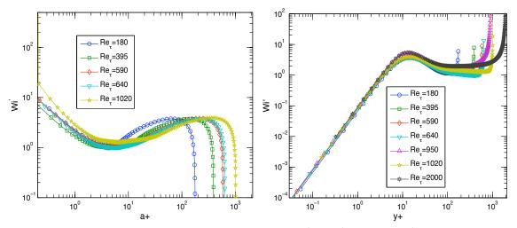
Figure 3. The distributions of Weissenberg number  $Wi' = \lambda' a^+$  vs.  $a^+$  (a) and vs.  $y^+$  (b) in log-log plot.
