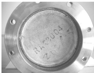
Figure 3: The catalytic converter without cover. This picture shows the exit side of the honeycomb. Velocity profiles were analyzed on this side.
