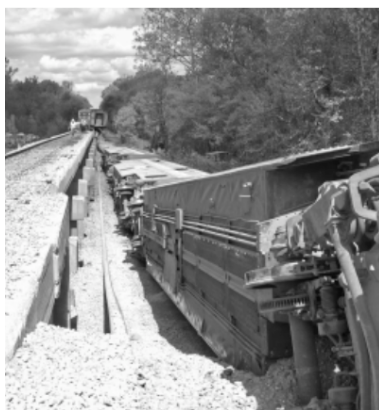
Figure 1. Derailment caused by failure on bolted joints
