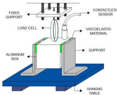
Figure 1. Experimental setup for characterizing the viscoelastic material.
