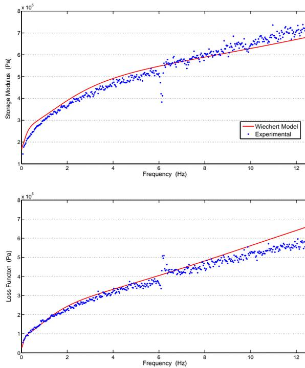
Figure 3. Storage modulus and loss function: Experimental and predicted by the Wiechert model.
