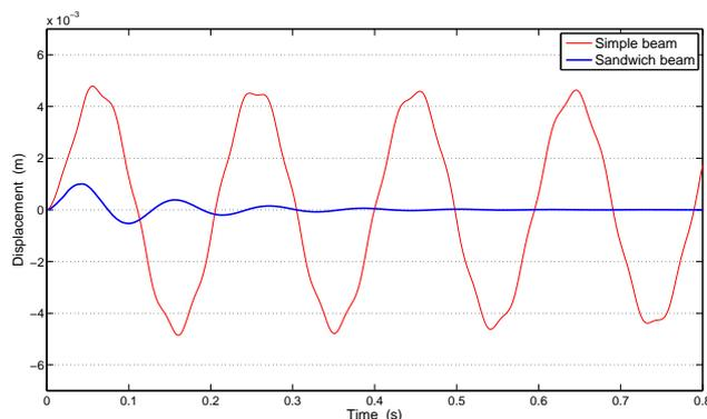
Figure 5. Displacement at the free end of the simple and sandwich beams due to an impulsive excitation.
