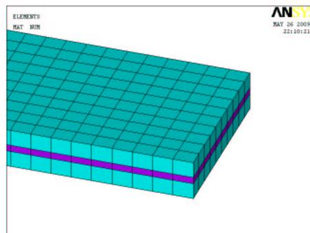
Figure 4. Finite element mesh at the free end of the sandwich beam.
