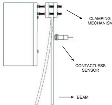
Figure 2. Experimental setup for determining the modal properties of the simple and sandwich beams.
