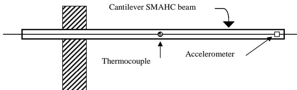
Figure 1. Schema of the experimental assembler for measurements of the natural frequency of SMAHC beam specimen.
