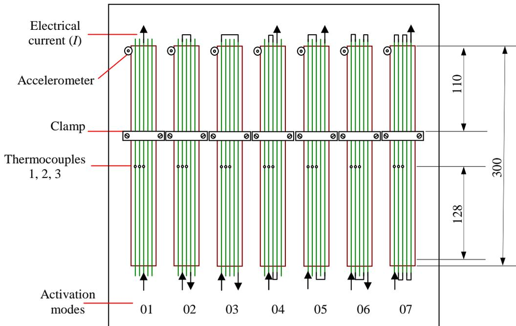
Figure 5. Different modes for electrical activation of the SMAHC beam specimen.
