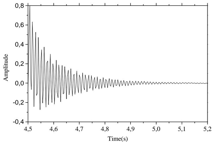
Figure 7. Time response of the SMAHC beam to a pulse impact without any activated SMA wire (room temperature).
