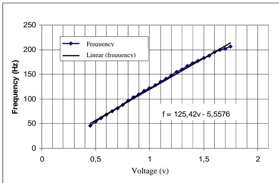
Figure 4. Relation between frequency and voltage of the DC electrical motor.
