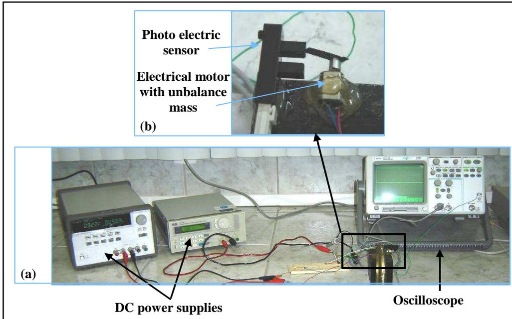
Figure 3. Assembly for the motor characterization used as electromechanical driver (small shaker). (a) General view of the developed assembly. (b) Detail of the photoelectric sensor and motor.
