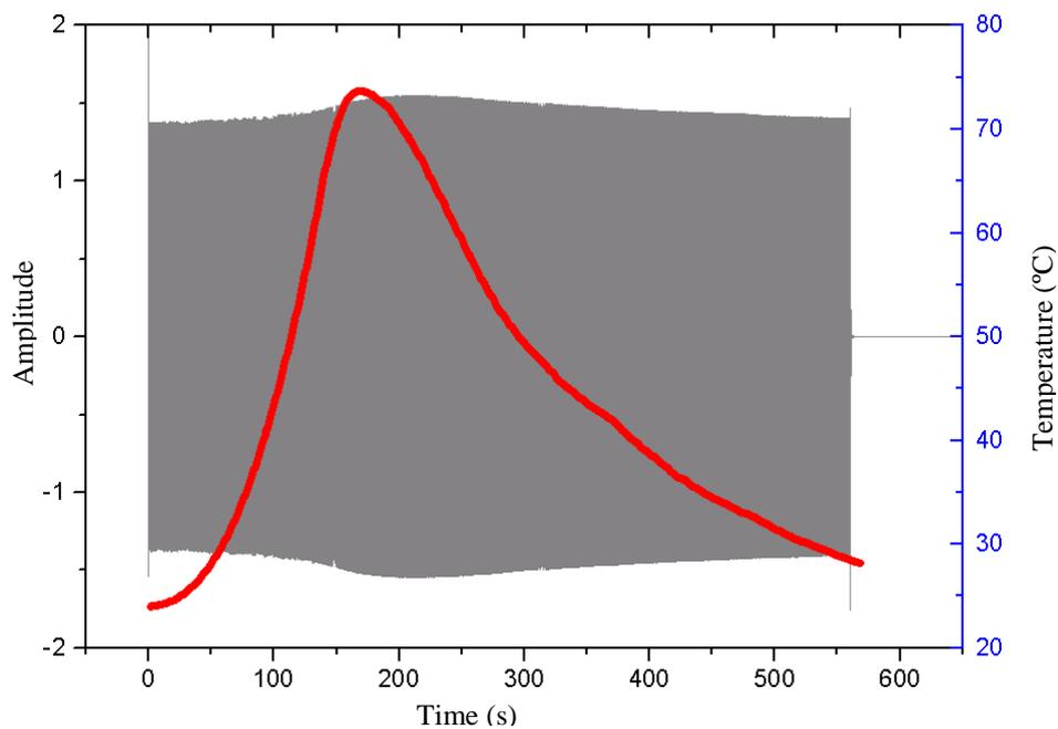
Figure 10. Amplitude response as a function of time for small shaker below the resonance frequency with activation mode 05 and evolution of the temperature of the SMAHC beam.
