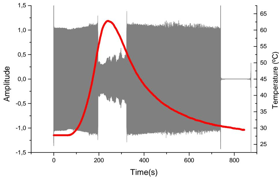
Figure 9. Amplitude response as a function of time for small shaker in the resonance frequency with activation mode 05 and evolution of the temperature of the SMAHC beam.
