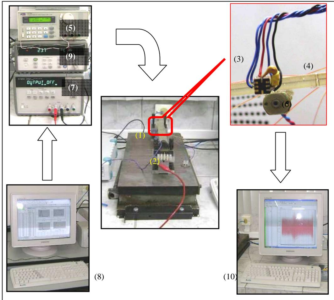
Figure 6. Experimental set-up for the SMAHC beam dynamic response.
