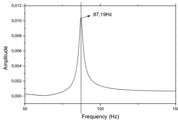
Figure 8. FFT of the voltage time signal shown in Fig 7.
