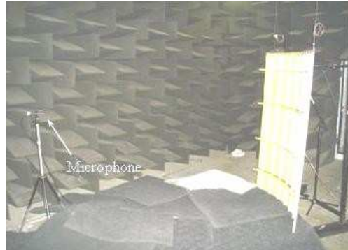
Figure 5. Driven panel inside the semi-anechoic chamber.
