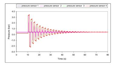
Figure 4. Numerical results in a pipeline without leak.
