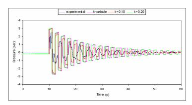
Figure 7. Comparison between numerical and experimental results in the pipeline without leak.
