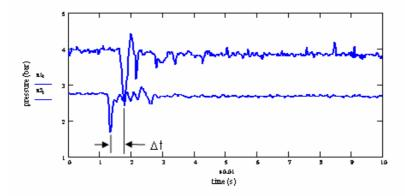
Figure 1. Characteristic pressure waveforms during a simulated leak test.
