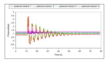
Figure 3. Experimental results in a pipeline without leak.
