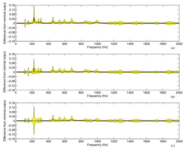
Figure 6. Difference from nominal model of filter output mean and confidence intervals for the isolation of first (a), second (b) and third (c) modes.
