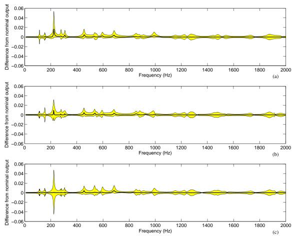
Figure 5. Difference from nominal model of filter output mean and confidence intervals for the isolation of first (a), second (b) and third (c) modes.
