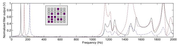
Figure 2. Normalized output of the modal filter designed for the isolation of the first three vibration modes.
