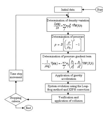
Figure 5. Algorithm of SPH method
