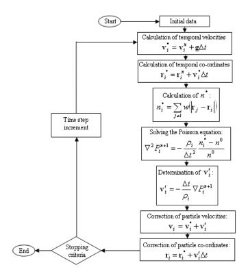
Figure 3. Algorithm of MPS method
