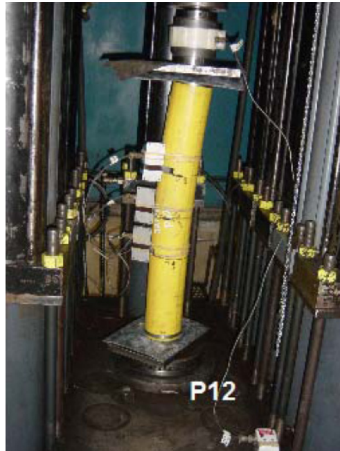
Figure 6. Compressive Testing of Umbilicals (test setup)
