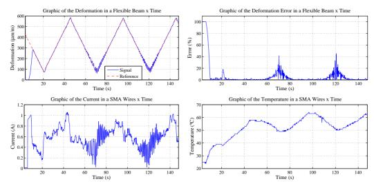
Figure 13. Deformation behavior, current, error and temperature for a triangular reference of 20 mHz in the presence of an external disturbance of 3.5 Hz.
