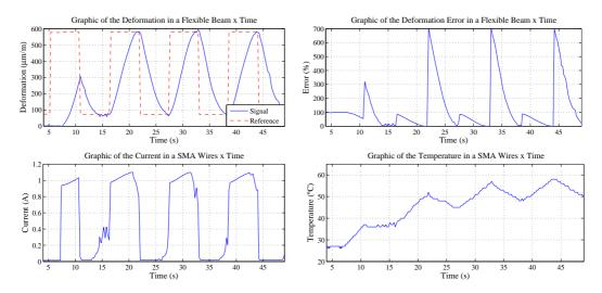
Figure 6. Deformation behavior, current, error and temperature for a squared reference of 90 mHz in the absence of external disturbance.
