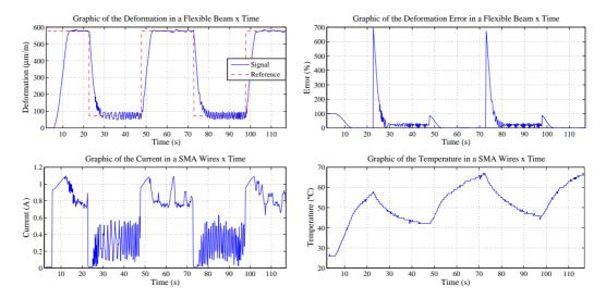
Figure 11. Deformation behavior, current, error and temperature for a squared reference of 20 mHz in the presence of an external disturbance of 3.5 Hz
