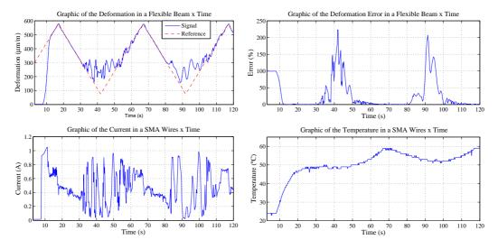
Figure 15. Deformation behavior, current, error and temperature for a triangular reference of 20 mHz in the presence of an external disturbance of 4.5 Hz.
