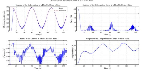
Figure 12. Deformation behavior, current, error and temperature for a sinusoidal reference of 20 mHz in the presence of an external disturbance of 3.5 Hz.
