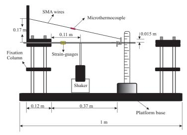
Figure 1. Schematic diagram of the developed experimental platform.
