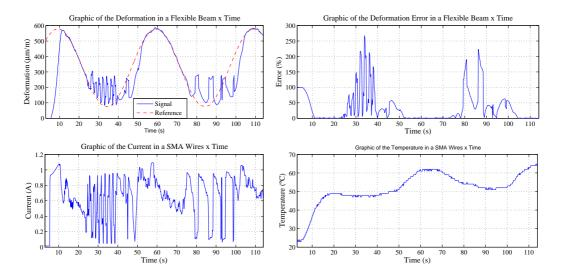
Figure 14. Deformation behavior, current, error and temperature for a sinusoidal reference of 20 mHz in the presence of an external disturbance of 4.5 Hz.
