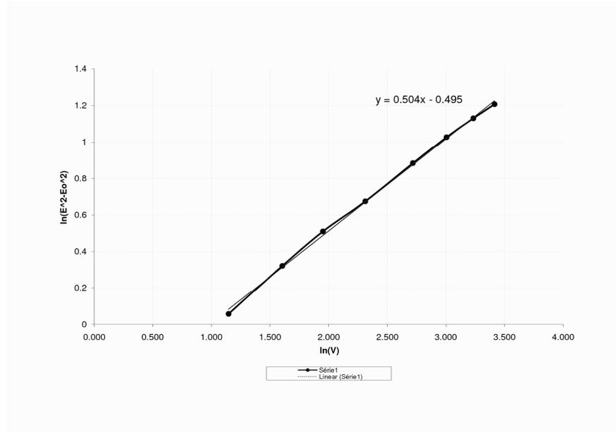
Figure 2 - Response curve of the anemometer.
