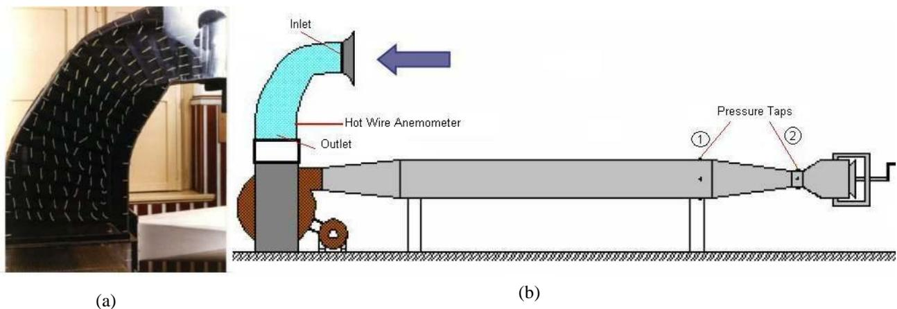
Figure 3 - (a) View of the Test Section (b) Schematic representation of the complete test apparatus.
