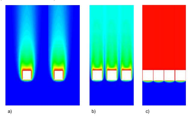
Figure 4. Temperature distribution as function of the spacing between square cylinders ( $\tilde{s}_0$ ): a) long distance; b) intermediate distance (optimal configuration) and c) short distance
