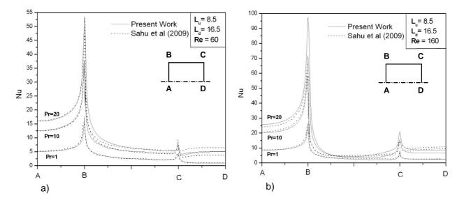
Figure 2. Local Nusselt number obtained from the present code and that presented in Sahu *et al.* (2009) for flow with various Prandtl numbers, Pr = 1, 10 and 20, and a fixed Reynolds number – a) Re = 60 and b) Re = 160
