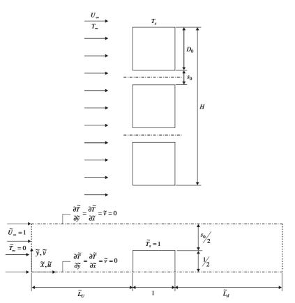
Figure 1. Parallel square cylinders arrange and the computational domain
