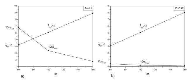
Figure 6. Dimensionless optimal heat transfer rate ( $\tilde{q}_{opt}$ ) and dimensionless optimal spacing between square cylinders ( $\tilde{s}_{0,opt}$ ) as function of Reynolds numbers for Prandtl numbers: a) Pr = 0.1 and b) Pr = 0.72
