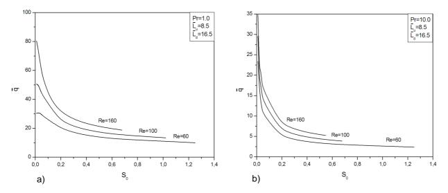
Figure 5. Optimization of dimensionless heat transfer rate ( $\tilde{q}$ ) as function of the dimensionless distance between the square cylinders ( $\tilde{s}_0$ ) for various Reynolds numbers, Re = 60, 100 and 160, and Prandtl numbers: a) Pr = 1.0 and b) Pr = 10.0
