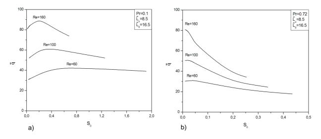
Figure 3. The optimization of dimensionless heat transfer rate ( $\tilde{q}$ ) as function of the dimensionless distance between the square cylinders ( $\tilde{s}_0$ ) for various Reynolds numbers, Re = 60, 100 and 160, and Prandtl numbers: a) Pr = 0.1 and b) Pr = 0.72
