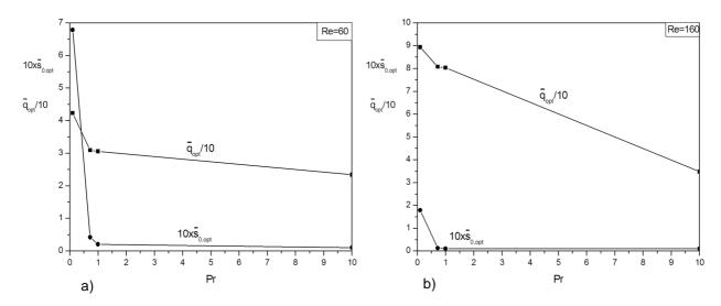
Figure 7. Dimensionless optimal heat transfer rate ( $\tilde{q}_{opt}$ ) and dimensionless optimal spacing between square cylinders ( $\tilde{s}_{0.opt}$ ) as function of Prandtl numbers for Reynolds numbers: a) Re = 60 and b) Re = 160
