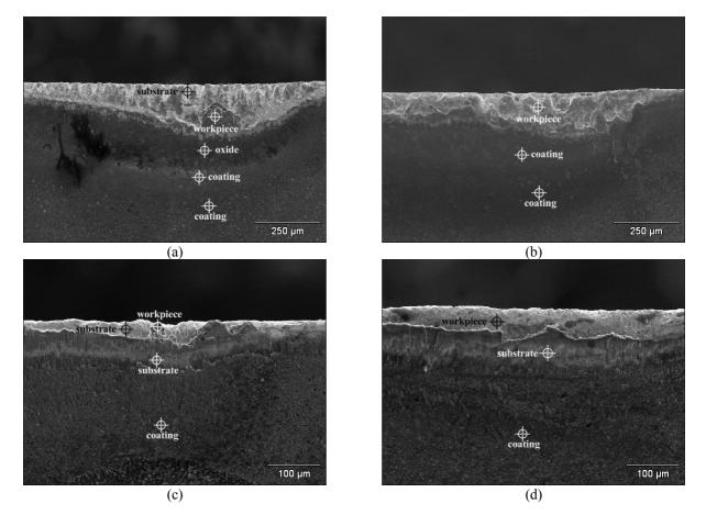
Figure 2. SEM pictures of worn tools as a function of cooling-lubrication condition: (a) flood, (b) MQL, (c) air and (d) dry
