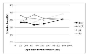
Figure 4. Microhardness depth profile as a function of cooling-lubrication condition
