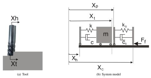
Figure 1. Tool and system modeling
