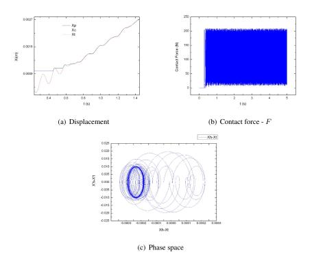
Figure 5.  $v_f = 2$ mm/s,  $\tau_s = 100$ MPa and w = 1800rpm
