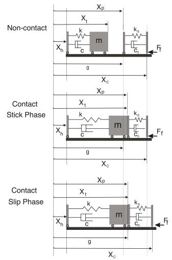
Figure 2. Contact / Non-contact situations
